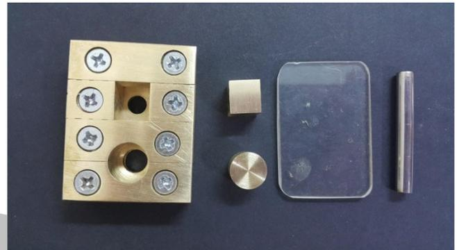
Fig.2: Split copper mold for fabricating wax specimens.
