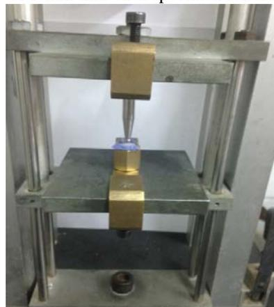
**Figure 2:** Biaxial flexural strength test set up.
